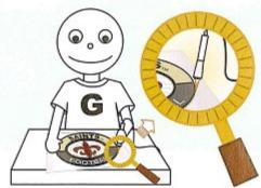
8. 使用電熱刀將徽章與多餘的膠膜分離。 Separate the extra film by a hot cutter.
